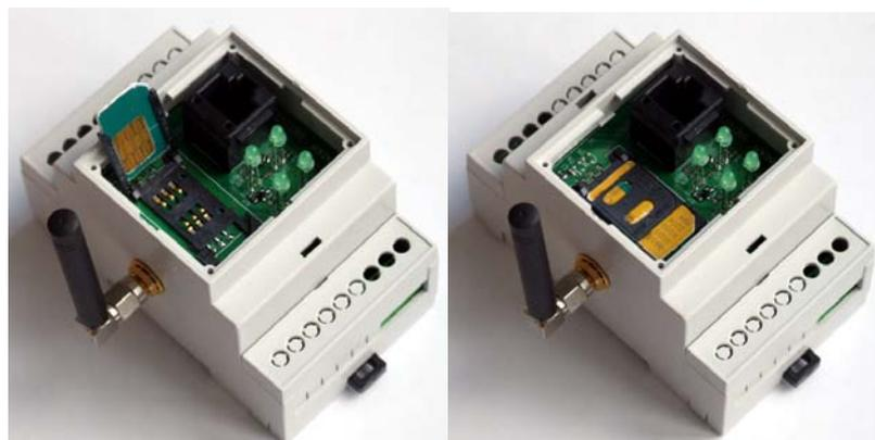
Picture 3. Inserting SIM card
